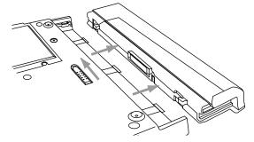
Figure 2-2 Removing the Battery
